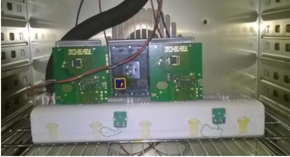
Figure 5: The three samples in the oven for high temperature test.
